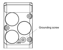
The PSD4xx must be grounded before the power supply cable is connected. The grounding cable must be connected to the correct position on the PSD4xx and to the ground potential (e.g. machine base).
