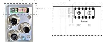
Note: If these address switches are set to 00, the address can be set via the CAN bus with SDO #2026.
