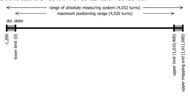
Note: The numerator factor and denominator factor can be used to map any spindle resolutions. Using the referencing value, you can shift the whole range of values.
